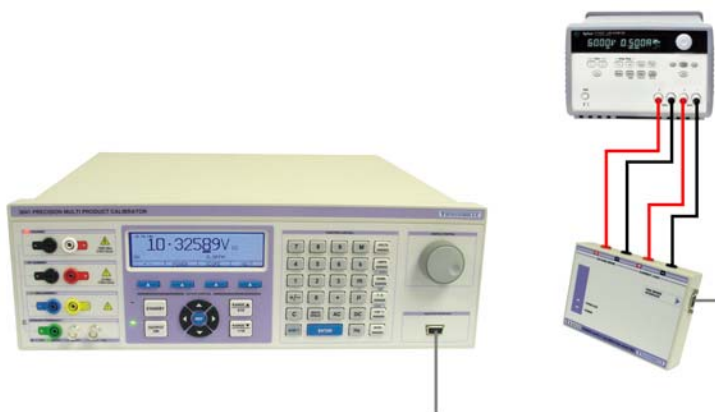
Fig. 2 : 4 Terminal Power Supply Connection Example
