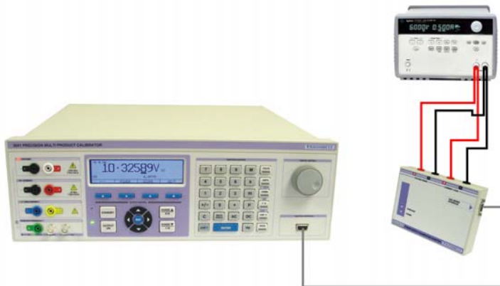
Fig. 1 : 2 Terminal Power Supply Connection Example
