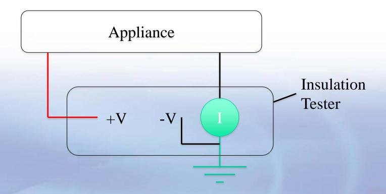
Basic Block Diagram of Insulation Tester
